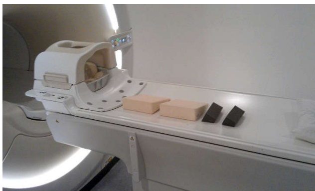
Fig. 20: Items needed for QA tool for Stability, Ingenia system.
