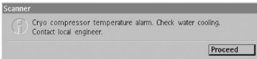
Fig. 13: Cryo compressor temperature alarm. Check water cooling. Contact local engineer.
