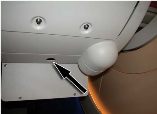
Fig. 6: Manual override switch.
